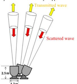
The Doppler SODAR that we will be installing is a device that sends out sound waves from three transmitter/receivers, and measures the discrepancy between the frequencies of the transmitted waves and the scattered waves that are received in order to measure wind direction and wind speed in the upper air. The Doppler SODAR makes it possible to measure meteorological conditions in the upper air using a device positioned on the ground.
