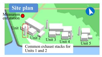
A measurement station used for obtaining meteorological data that is representative of the entire facility is located within the grounds of the power station, and we intend to install the Doppler SODAR on this measurement station.
