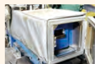
Induction-heater for rubber extrusion dies
