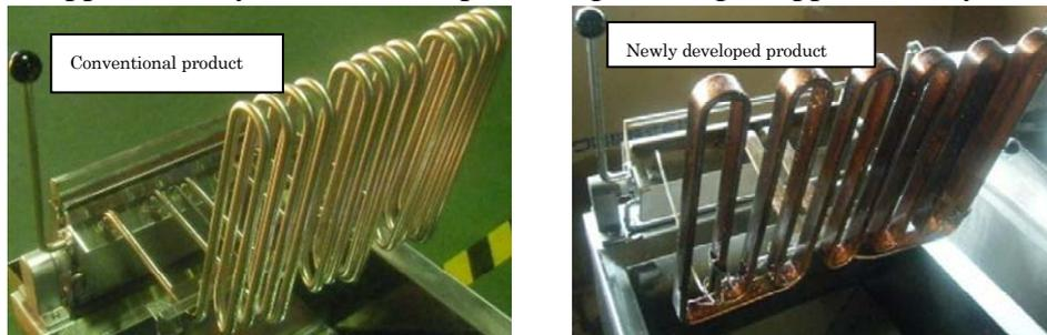
Figure 3 : Comparison of heating mechanism
