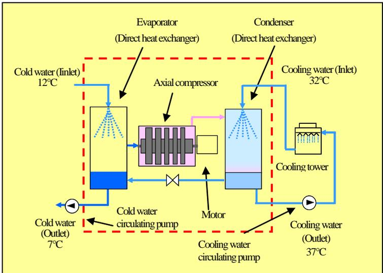
Water acting as refrigerant circulates from the evaporator to the axial compressor, then to the condenser and back to the evaporator, while being mixed with cooling water and cold water.
