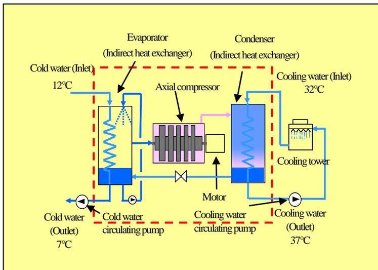
Water acting as refrigerant circulates from the evaporator to the axial compressor, then to the condenser and back to the evaporator (the refrigerant for this section has been switched from fluorocarbon to water).
