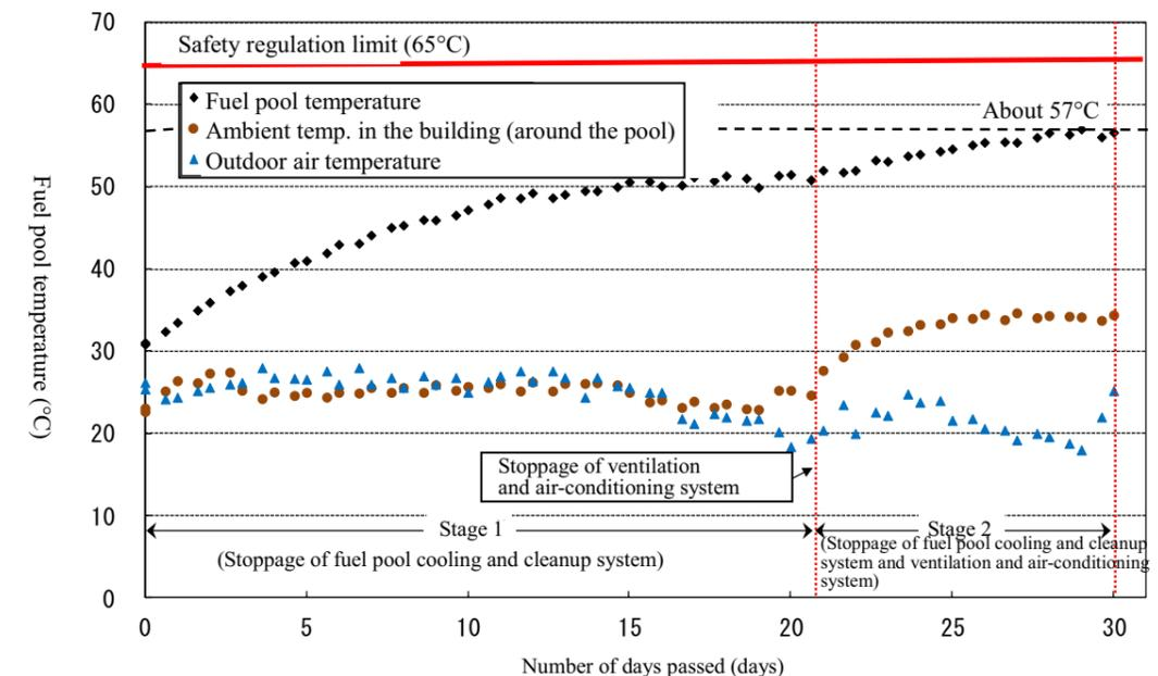
Figure 1. Results of fuel pool water temperature measurement (September 6 – October 6, 2011)
