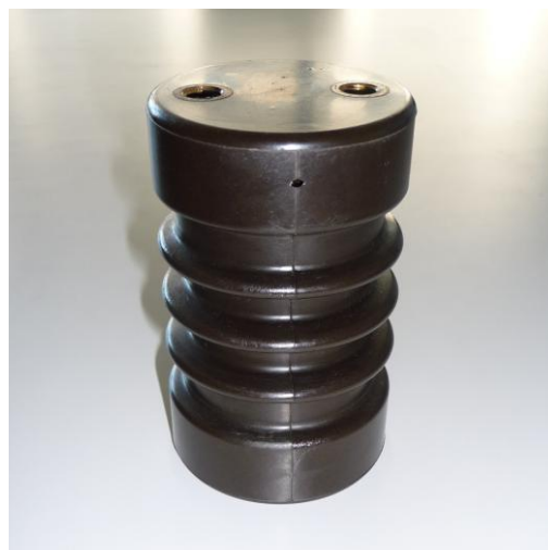
Photo 1: Example of a product (cubicle insulator) made with the developed resin
