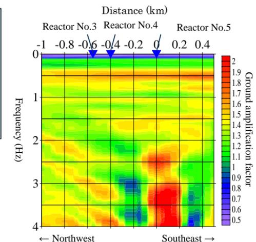
In the vicinity of Reactor No. 5, the ground amplification factor was higher, and a difference in tremors was observed.
