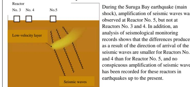
The results of an analysis using a ground model that reflected the distribution of this "low-velocity layer" showed that in the case of the tremors from the direction of the main shock of the Suruga Bay earthquake, a difference was observed in the vicinity of Reactor No. 5.
