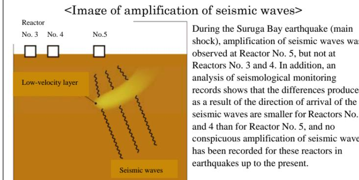
The results of an analysis using a ground model that reflected the distribution of this "low-velocity layer" showed that in the case of the tremors from the direction of the main shock of the Suruga Bay earthquake, a difference was observed in the vicinity of Reactor No. 5.
