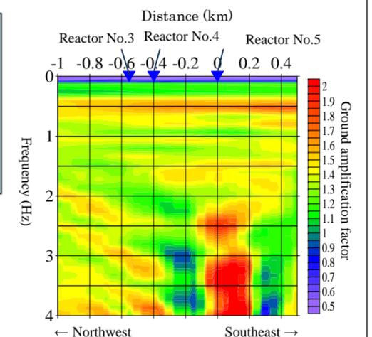
In the vicinity of Reactor No. 5, the ground amplification factor was higher, and a difference in tremors was observed.
