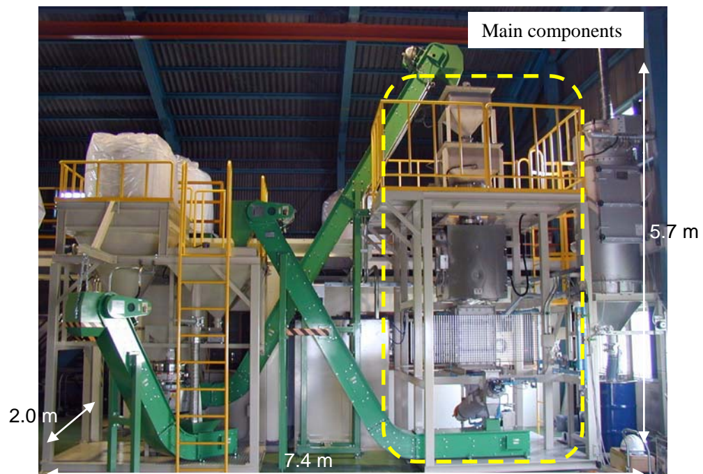
Figure 2 External view of halon decomposer
