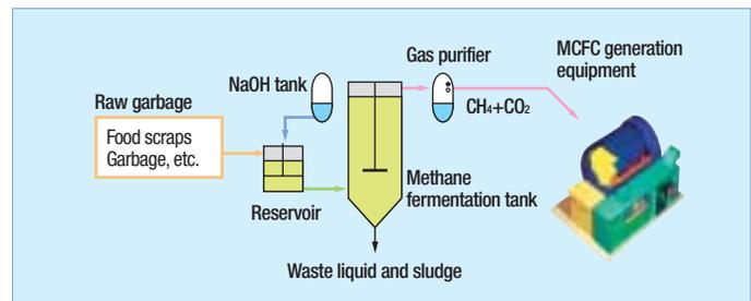
Verification test of fuel-cell power generation at Expo 2005
