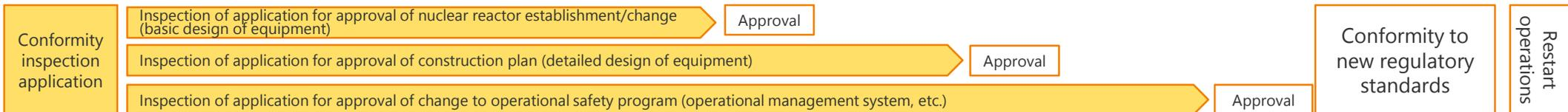
**Main inspection items and progress of application for approval of nuclear reactor establishment/change**
