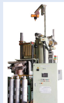
Arc-type ladle heating system adopted by Aishin Takaoka
