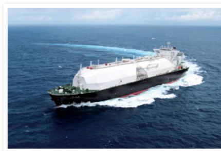
▲ A new LNG carrier with a pea-pod-shaped shell
